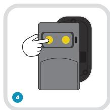
Place the original remote if possible, back to back, press the button on the original you want to copy until the LED on the A3 turns on, then release the buttons.
