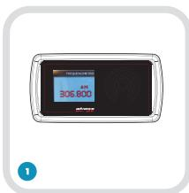
With the help of a frequency meter, adjust the frequency of the A3 to match the frequency of the original remote.
